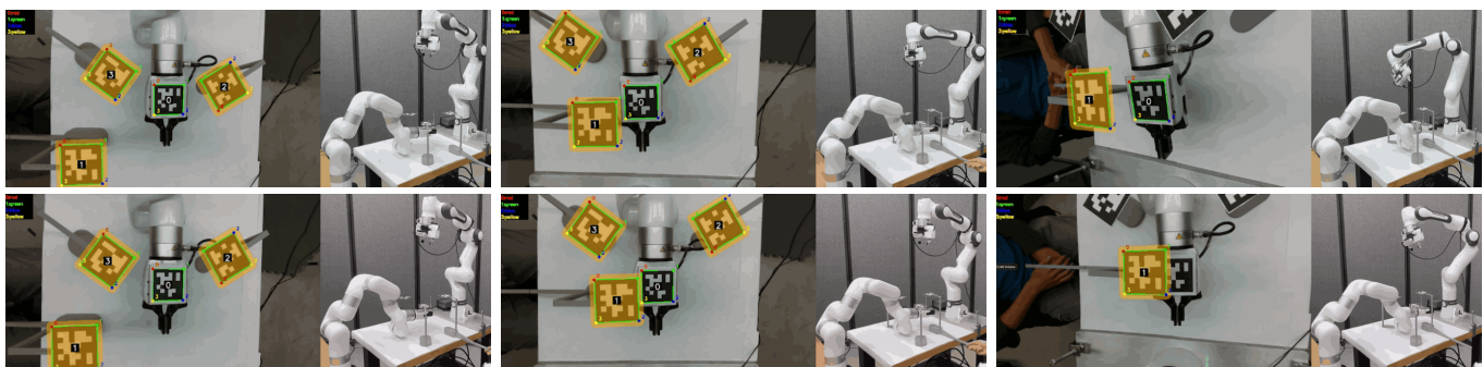
(d) Scenario 4 with one dynamic occluding objects: hierarchical controller (top row) versus MPC alone (bottom row)
